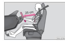
Fig. 102 The correct distance of the driver from the steering wheel
