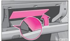
Fig. 75 Storage compartment: tiltable partition wall
