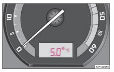
Fig. 8 Multi-functional indicator: the outside temperature
