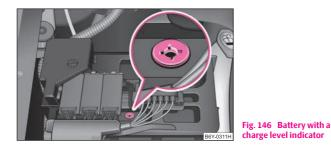
There is a so-called magic eye  $\Rightarrow$  fig. 146 located on the top of the battery. The "magic eye" changes its colour in line with the charge state of and electrolyte level in the battery.
