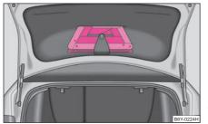
Fig. 151 Placing of the warning triangle in the boot lid (on a sedan)
