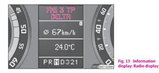
These displays appear in addition to the normal information in the radio display.
