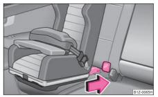
Fig. 129 The ISOFIX child seat is pushed into the mounting funnels
