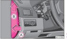
Fig. 165 Left side of the dash panel: fuse cover
