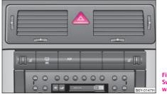
Fig. 35 Dash panel: Switch for hazard warning lights
