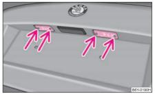
Fig. 178 Remove the licence plate light
