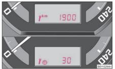
Fig. 5 Service Interval Display
