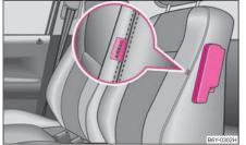
Fig. 117 Driver seat: Installation position of airbag
