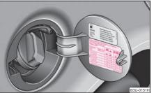
Fig. 148 An opened fuel filler flap with the tyre inflation pressure table
