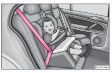
Fig. 125 Child seat with padded table in Group 1 installed on rear seat bench facing the direction of travel
