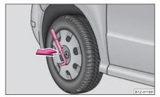
Fig. 155 Removing the full wheel trim
