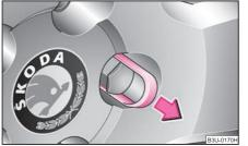
Fig. 157 Changing a wheel: Removing the cap
