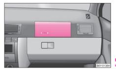
Fig. 114 Front passenger airbag in the dash panel
