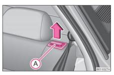
Fig. 52 Unlock the seat backrest
