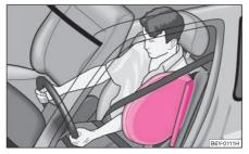
Fig. 118 Side airbags deployed
