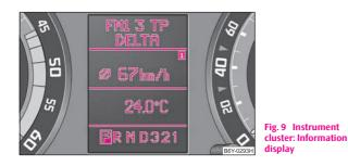
The information display provides you with information in a convenient way concerning the **current operating state of your vehicle**. The information system also provides you with data (depending on the equipment installed in the vehicle) relating to the radio, multi-functional indicator, navigation system and automatic gearbox.
