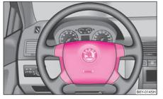
Fig. 113 Driver airbag in the steering wheel
