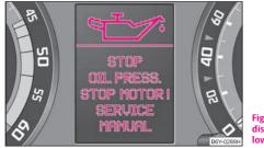
Fig. 14 Information display: Oil pressure is low
