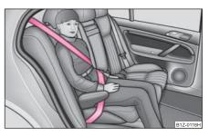
Fig. 127 Child seat in Group 3 installed on the rear seat facing the direction of travel
