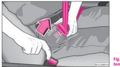
Fig. 110 Releasing lock tongue from belt lock
