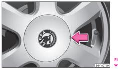
Fig. 156 Pulling off the wheel trim cap
