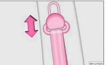
Fig. 109 Front seat: Seat belt height adjuster
