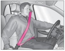
Fig. 107 Routing of webbing over the shoulders and the lap belt
