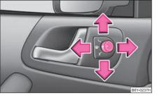
Fig. 45 Inner part of door: Rotary knob
