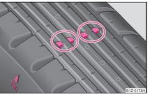
Fig. 149 Tyre tread with wear indicators
