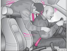
Fig. 106 The rear seat occupant is thrown forward if not wearing a belt
