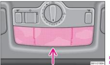
Fig. 177 Remove interior light
