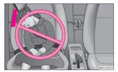
Fig. 122 Seated position of an unprotected child at risk from side airbag
