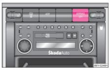
Fig. 120 Indicator light for a switched off front seat passenger airbag
