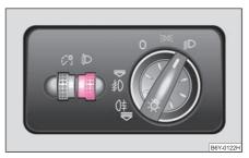
Turn the control dial ⇒ page 44, fig. 34 until you have adjusted the low beam so that oncoming traffic is not dazzled.
