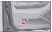
Fig. 39 Front door: Warning light The warning light is located in the door trim panel below  $\Rightarrow$  page 47, fig. 39.
