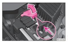
Fig. 145 The battery: Open up the cover
