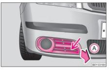
Fig. 162 Front bumper: Protective grille
