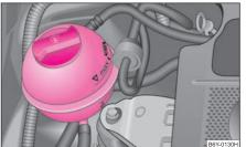
Fig. 143 Engine compartment: Coolant expansion bottle
