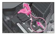
Fig. 167 The battery: Opening of the positive terminal cover.
