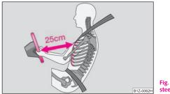
Fig. 116 Safe distance to steering wheel
