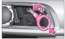
Fig. 163 Front bumper: Installing the towing eye
